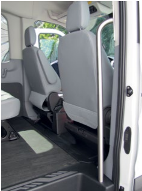
Grab bar – add at entrance on Rightside (B-Pillar) or Leftside (C-Pillar). Overhead grab bars available too!
